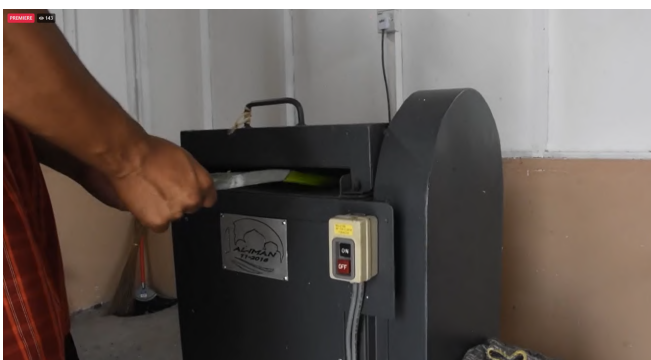
Mechanism used to extract the fiber from the pineapple leaves.
