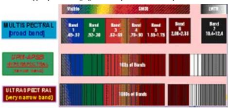
Comparison between multispectral, hyperspectral, and ultraspectral bands (Image courtesy of Dr. Kamaruzaman)
