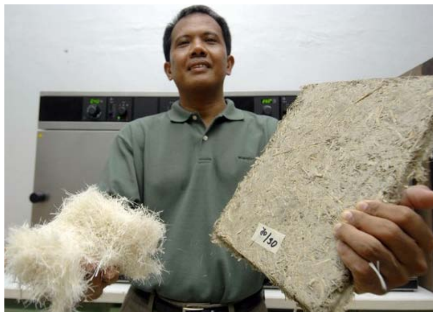
UPLB Professor Menandro N. Acda displays processed chicken feathers on left and a board composed of a mixture of feathers and cement at his laboratory in Los Baños, Laguna, Philippines on 30 July 2008. (Photo source: Getty Images)
