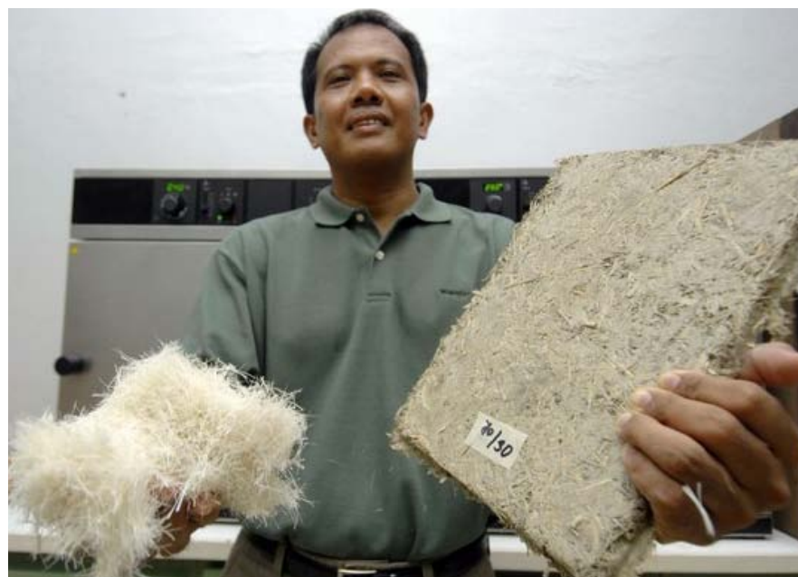
UPLB Professor Menandro N. Acda displays processed chicken feathers on left and a board composed of a mixture of feathers and cement at his laboratory in Los Baños, Laguna, Philippines on 30 July 2008. (Photo source: Getty Images)
