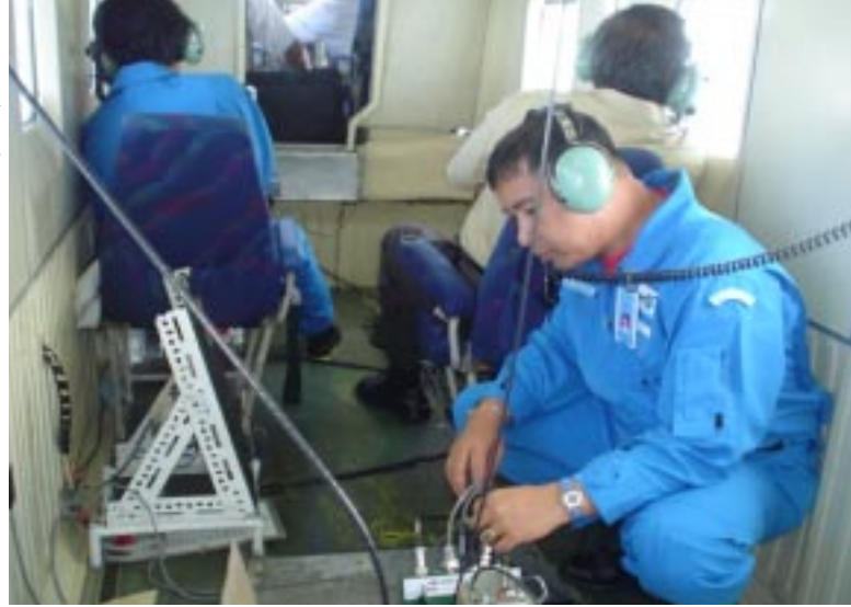
Dr. Kamaruzaman mounts a complete UPM-Aeroscan's AISA sensor system on a Sabah Air GAF Nomad N22B, the small aircraft used by his team to conduct airborne hyperspectral imaging. (Photo courtesy of Dr. Kamaruzaman)
